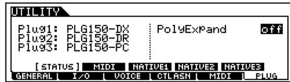
In the examples used for the screen shots in this article the PLG150-DR board is in Plugin Slot 2 and the PLG150-PC board is in Plugin Slot 3. (A PLG150-DX is in slot 1). \*Note: PLG150 boards can go in any slot, no restrictions.
