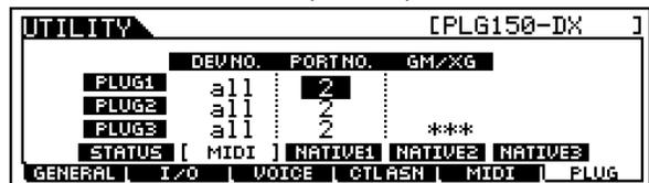
This would allow you to break the 16-channel limit. You can select the Port assignment for each board in UTILITY/ F6 PLG/ SF2 MIDI. The host (Motif or S90) remains fixed at PORT 1 – you cannot change this assignment. Additionally, when using the USB Port in this fashion you can send an additional PORT out the MIDI OUT jack of the Motif/S90. Under the MIDI IN/OUT parameter where you select USB (UTILITY/ F5 MIDI/ SF4 Other) you will find the “ThruPort” parameter –
