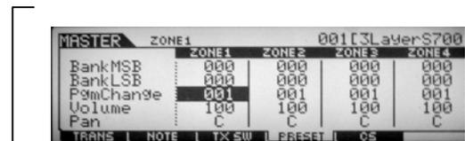
F5 Selects the CS or Control Slider display. On a per-zone basis you can set the controller transmitted by each of the 4 CS sliders when they are in their zone control function setting (last row down on the Control Slider area on the right of the keyboard front panel)
