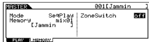
The ever-important zone switch is on the right side of the screen. **To get to the master keyboard control functions this switch must be set to ON. To do this, use the cursor controls and press the [INC/YES] button.** You should see the screen below:
