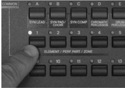
You have a total of 4 zones that can be called up for editing. **After you have set the Zone Switch to on, press the EDIT button, then press Buttons 1, 2, 3 or 4 (ELEMENT/PERF PART/ZONE) on the right hand side of the keyboard to bring up the zone edit screen.**
