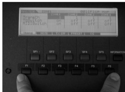
Navigating through the various screens is done via the function keys located directly beneath the screen. F1, F2, F3, F4 and F5 are active in the Zone edit screen.
