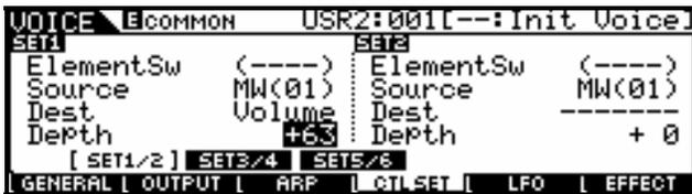
In the above example, the Volume parameter is 'common' to **all Elements**. We know this because the Element Switches are grayed out (parenthesis). If you were to activate additional Elements they would also share the same setting when you select a 'common' destination. The modulation wheel will effect all the Elements. The +63 Depth setting sets the maximum range of the controller. Try it...move the mod wheel...
