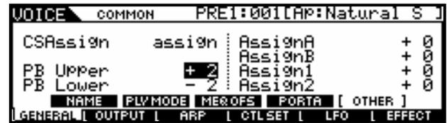
The Pitch Bend wheel actually sends out 16,384 different units, how far this bends the pitch is always determined in the receiving device. While raising the pitch bend wheel in the screen shot above will raise the pitch two half steps, out via MIDI a receiving module might see this as an octave or a fifth (how far the PB changes is always determined in the receiving device).
