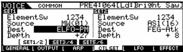
Above you see a typical synth lead Voice PRE4:064 [Ld:Bright Saw]. A two Element Voice that has the Mod Wheel as the ELFO-PM depth control – this translates to Element Low Frequency Oscillator- Pitch Modulation control. Depth = +27. As you move the wheel up you will add vibrato (pitch modulation) to the Voice
