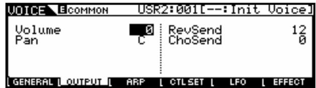
Now when you move the modulation wheel you have **total** control over the volume of the Voice. The position of the modulation wheel is now an **absolute** representation of the current common volume, 0-127. We call this process 'biasing' the parameter (in this case, volume) to the controller. In other words, it will now look to this controller (mod wheel) for volume instructions.
