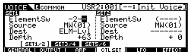
And in a similar fashion to before, you would need to set the initial level of the Element(s) that you are controlling to zero (bias its level to the MW). Instead of "Total Voice Volume" we are looking for the level of this particular Element. This is found on the Element Amplitude page: Return to Element Level editing by pressing program button [2] (Element 2 Select)
