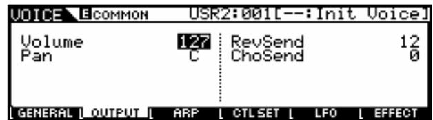
Similarly, a volume assignment can be made on the Element level. This would allow the player/programmer to have control over specific parts of the sound (Elements) within a Voice. In our Control Set instead of making the Destination = Volume (common overall volume) like before, this time assign it to **ELM-Lvl** or Element Level. When ELM-Lvl is selected you can individually assign which elements will respond to this Control Set's Depth setting when the physical controller is moved.
