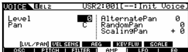
When you set Element 2's Level to 0, it is biased to the MW. This is a very flexible arrangement. You can expand upon it and dream up your own configurations. For example, you could take Control Set 2 and program it to control just Element 1 with the same Mod Wheel but set the ELM-Lvl DEPTH to -64. Now when you move the wheel it will fade out one sound and fade in the other.
