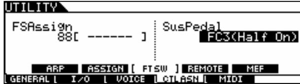
The "SusPedal" parameter selects the Foot Controller type connected to the FOOTSWITCH SUSTAIN jack.
