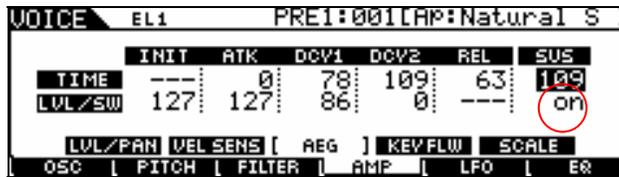
From this display you can make all the time and level settings for the Amplitude EG, which determine how the volume of the sound changes over time. These can be used to control the change in volume from the moment a note is pressed on the keyboard to the moment the sound stops. The full names of the available parameters are shown in the chart below, as they appear in the display.
