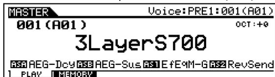
Any time MASTER 001 is recalled it will recall your "3LayerS700" sound. There is no signal assigned to go out via MIDI so any connected modules will be silent.
